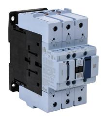
WEG Electric CWB series IEC contactor, 95A, (3) N.O. power poles, (1) N.O./(1) N.C. auxiliary contacts, 24 VAC (50/60Hz) coil voltage.
