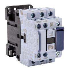
WEG Electric CWB series IEC contactor, 9A, (3) N.O. power poles, (1) N.O./(1) N.C. auxiliary contacts, 208-240 VAC (60Hz)/180-208 VAC (50Hz) coil voltage.
