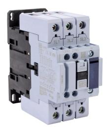
WEG Electric CWB series IEC contactor, 80A, (3) N.O. power poles, (1) N.O./(1) N.C. auxiliary contacts, 480 VAC (50/60Hz) coil voltage.
