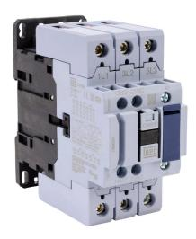
WEG Electric CWB series IEC contactor, 80A, (3) N.O. power poles, (1) N.O./(1) N.C. auxiliary contacts, 120 VAC (50/60Hz) coil voltage.
