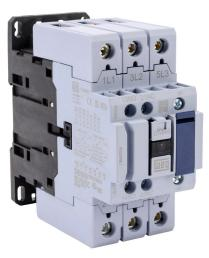
WEG Electric CWB series IEC contactor, 65A, (3) N.O. power poles, (1) N.O./(1) N.C. auxiliary contacts, 208-240 VAC (60Hz)/180-208 VAC (50Hz) coil voltage.
