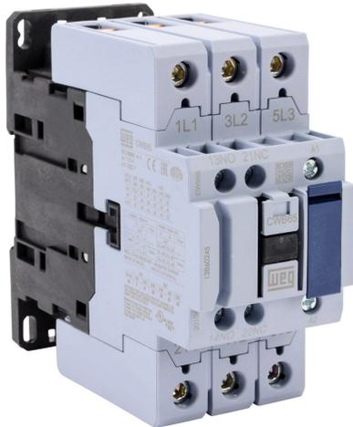
WEG Electric CWB series IEC contactor, 65A, (3) N.O. power poles, (1) N.O./ (1) N.C. auxiliary contacts, 120 VAC (50/60Hz) coil voltage.
