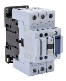
WEG Electric CWB series IEC contactor, 50A, (3) N.O. power poles, (1) N.O./(1) N.C. auxiliary contacts, 120 VAC (50/60Hz) coil voltage.
