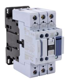
WEG Electric CWB series IEC contactor, 40A, (3) N.O. power poles, (1) N.O./(1) N.C. auxiliary contacts, 208-240 VAC (60Hz)/180-208 VAC (50Hz) coil voltage.
