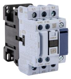
WEG Electric CWB series IEC contactor, 38A, (3) N.O. power poles, (1) N.O./(1) N.C. auxiliary contacts, 208-240 VAC (60Hz)/180-208 VAC (50Hz) coil voltage.
