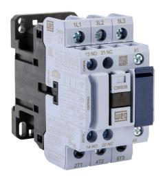
WEG Electric CWB series IEC contactor, 38A, (3) N.O. power poles, (1) N.O./(1) N.C. auxiliary contacts, 480 VAC (50/60Hz) coil voltage.
