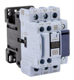
WEG Electric CWB series IEC contactor, 38A, (3) N.O. power poles, (1) N.O./(1) N.C. auxiliary contacts, 120 VAC (50/60Hz) coil voltage.
