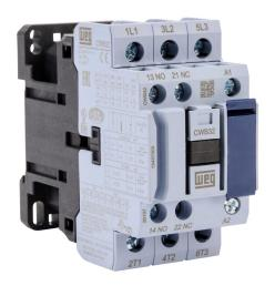
WEG Electric CWB series IEC contactor, 32A, (3) N.O. power poles, (1) N.O./(1) N.C. auxiliary contacts, 208-240 VAC (60Hz)/180-208 VAC (50Hz) coil voltage.
