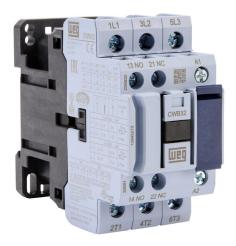
WEG Electric CWB series IEC contactor, 32A, (3) N.O. power poles, (1) N.O./(1) N.C. auxiliary contacts, 120 VAC (50/60Hz) coil voltage.
