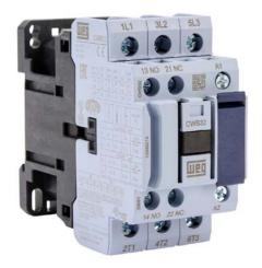
WEG Electric CWB series IEC contactor, 32A, (3) N.O. power poles, (1) N.O./(1) N.C. auxiliary contacts, 120 VAC (50/60Hz) coil voltage.
