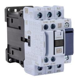
WEG Electric CWB series IEC contactor, 32A, (3) N.O. power poles, (1) N.O./(1) N.C. auxiliary contacts, 24 VDC coil voltage.
