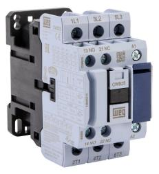
WEG Electric CWB series IEC contactor, 25A, (3) N.O. power poles, (1) N.O./(1) N.C. auxiliary contacts, 120 VAC (50/60Hz) coil voltage.
