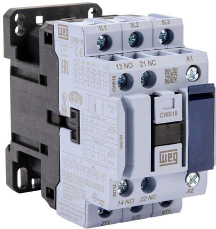
WEG Electric CWB series IEC contactor, 18A, (3) N.O. power poles, (1) N.O./ (1) N.C. auxiliary contacts, 208-240 VAC (60Hz)/180-208 VAC (50Hz) coil voltage.
