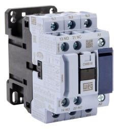
WEG Electric CWB series IEC contactor, 18A, (3) N.O. power poles, (1) N.O./(1) N.C. auxiliary contacts, 480 VAC (50/60Hz) coil voltage.
