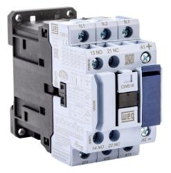
WEG Electric CWB series IEC contactor, 18A, (3) N.O. power poles, (1) N.O./(1) N.C. auxiliary contacts, 24 VDC coil voltage.
