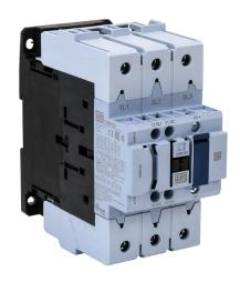
WEG Electric CWB series IEC contactor, 125A, (3) N.O. power poles, (1) N.O./(1) N.C. auxiliary contacts, 110-255 VAC/VDC coil voltage, electronic.
