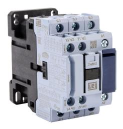
WEG Electric CWB series IEC contactor, 12A, (3) N.O. power poles, (1) N.O./(1) N.C. auxiliary contacts, 480 VAC (50/60Hz) coil voltage.
