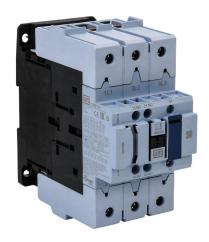
WEG Electric CWB series IEC contactor, 110A, (3) N.O. power poles, (1) N.O./(1) N.C. auxiliary contacts, 208 VAC (50/60Hz) coil voltage.
