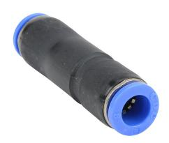
NITRA pneumatic push-to-connect fitting, union straight check valve, thermoplastic (PBT) body, (1) 5/16in (8mm) push-to-connect to (1) 5/16in (8mm) push-to-connect. Package of 5.
