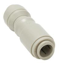
HydroMode potable water push-to-connect fitting, union straight check valve, acetal body, (2) 1/2in tube connection(s), NSF/ANSI 61. Package of 2.
