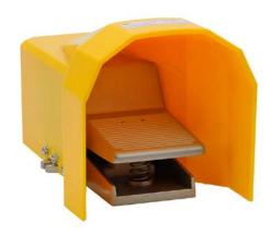
NITRA manual valve, 5-port (4-way), 2-position, locking foot pedal, detented, 1/4in female NPT inlet(s), 1/4in female NPT outlet(s), Cv=0.8.
