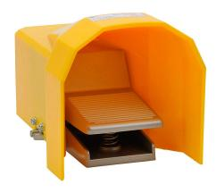
NITRA pneumatic manual valve, 5-port (4-way), 2-position, non-locking foot pedal, spring return, 1/4in female NPT inlet(s), 1/4in female NPT outlet(s), Cv=0.8.
