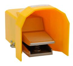
NITRA manual valve, 5-port (4-way), 2-position, non-locking foot pedal, spring return, 1/4in female NPT inlet(s), 1/4in female NPT outlet(s), Cv=0.8.
