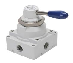
NITRA pneumatic manual valve, 4-port (4-way), 3-position, center closed, 4.4in handle, detented, 1/2in female NPT inlet(s), 1/2in female NPT outlet(s), Cv=5.29, through panel mount.
