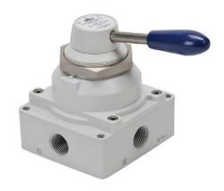
NITRA manual valve, 4-port (4-way), 2-position, 4in handle, detented, 1/2in female NPT inlet(s), 1/2in female NPT outlet(s), Cv=5.29, through panel mount.
