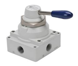
NITRA pneumatic manual valve, 4-port (4-way), 2-position, 4in handle, detented, 1/2in female NPT inlet(s), 1/2in female NPT outlet(s), Cv=5.29, through panel mount.
