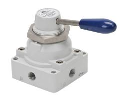
NITRA pneumatic manual valve, 4-port (4-way), 3-position, center closed, 4in handle, detented, 1/4in female NPT inlet(s), 1/4in female NPT outlet(s), Cv=0.89, through panel mount.
