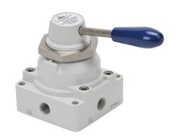
NITRA manual valve, 4-port (4-way), 3-position, center closed, 4in handle, detented, 1/4in female NPT inlet(s), 1/4in female NPT outlet(s), Cv=0.89, through panel mount.
