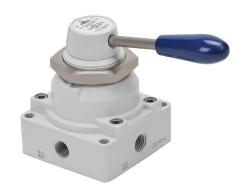
NITRA pneumatic manual valve, 4-port (4-way), 2-position, 4in handle, detented, 1/4in female NPT inlet(s), 1/4in female NPT outlet(s), Cv=0.89, through panel mount.
