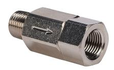
NITRA pneumatic threaded fitting, check valve, nickel-plated brass body, nickel-plated brass threads, (1) 1/8in male NPT to (1) 1/8in female NPT connection(s).
