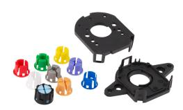
CUI Devices encoder accessory kit, replacement. For use with CUI Devices AMT11, AMT21 and AMT31 encoders. Includes (1) AMT standard base, (1) AMT standard wide base, and (1) AMT standard sleeve kit (9 sleeves sized from 2-8mm).
