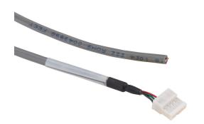
Same Sky encoder cable, 5-pin connector to pigtail, shielded, twisted pair, 6ft cable length. For use with Same Sky AMT103 encoders.
