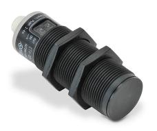
AutomationDirect capacitive proximity sensor, tubular, 30mm diameter x 90mm body, polybutylene terephthalate housing, N.O./ N.C. selectable output, 40mm sensing distance, non-flush, 10 Hz switching frequency, IP65 IP67, 1/2in - 20UNF thread.
