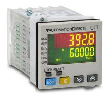
AutomationDirect multi-function digital counter/timer/ tachometer, two-line, 6-digit, two-color LCD, fully selectable timing range, 24 VDC operating voltage, (1) concurrent NPN transistor and SPST relay and (1) NPN transistor output(s), 1/16 DIN mount, screw terminal(s).
