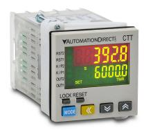
AutomationDirect multi-function digital counter/timer/tachometer, two-line, 6-digit, two-color LCD, fully selectable timing range, 100-240 VAC operating voltage, (1) concurrent NPN transistor and SPST relay and (1) NPN transistor output(s), 1/16 DIN mount.
