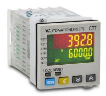
AutomationDirect multi-function digital counter/timer/tachometer, two-line, 6-digit, two-color LCD, fully selectable timing range, 100-240 VAC operating voltage, (1) concurrent NPN transistor and SPST relay and (1) SPDT relay output(s), 1/16 DIN mount, screw terminal(s).
