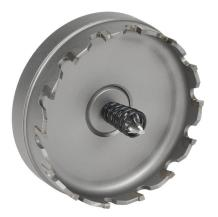
MK Morse hole cutter, 2-5/8in (67mm), carbide tipped steel, straight pitch, 3/16in (4.5mm) maximum cutting depth.
