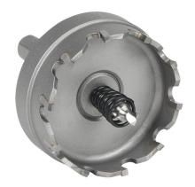
MK Morse hole cutter, 2in (51mm), carbide tipped steel, straight pitch, 3/16in (4.5mm) maximum cutting depth.
