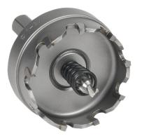
MK Morse hole cutter, 1-3/4in (44mm), carbide tipped steel, straight pitch, 3/16in (4.5mm) maximum cutting depth.
