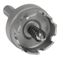
MK Morse hole cutter, 1-1/2in (38mm), carbide tipped steel, straight pitch, 3/16in (4.5mm) maximum cutting depth.
