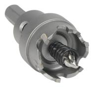
MK Morse hole cutter, 1-1/8in (29mm), carbide tipped steel, straight pitch, 3/16in (4.5mm) maximum cutting depth.
