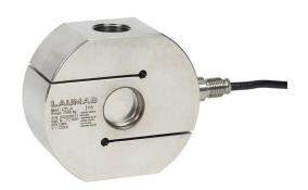
Laumas tension and compression load cell, 16530 lb/7500 kg, +/-0.02% of full scale accuracy, voltage signal range(s) of 2 mV/V, 3-15 VDC, stainless steel, IP68, 32.8ft/10m integral 6-wire shielded cable.
