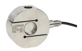
Laumas tension and compression load cell, 1102 lb/500 kg, +/-0.02% of full scale accuracy, voltage signal range(s) of 2 mV/V, 3-15 VDC, stainless steel, IP68, 32.8ft/10m integral 6-wire shielded cable.
