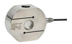
Laumas tension and compression load cell, 11020 lb/5000 kg, +/-0.02% of full scale accuracy, voltage signal range(s) of 2 mV/V, 3-15 VDC, stainless steel, IP68, 32.8ft/10m integral 6-wire shielded cable.
