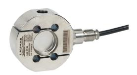
Laumas tension and compression load cell, 660 lb/300 kg, +/-0.02% of full scale accuracy, voltage signal range(s) of 2 mV/V, 3-15 VDC, stainless steel, IP68, 32.8ft/10m integral 6-wire shielded cable.
