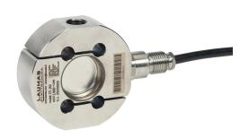
Laumas tension and compression load cell, 440 lb/200 kg, +/-0.02% of full scale accuracy, voltage signal range(s) of 2 mV/V, 3-15 VDC, stainless steel, IP68, 32.8ft/10m integral 6-wire shielded cable.
