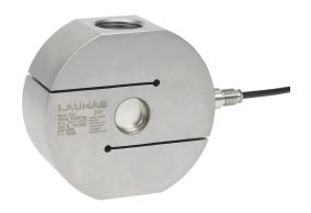
Laumas tension and compression load cell, 27550 lb/12500 kg, +/- 0.02% of full scale accuracy, voltage signal range(s) of 2 mV/V, 3-15 VDC, stainless steel, IP68, 32.8ft/10m integral 6-wire shielded cable.
