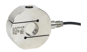
Laumas tension and compression load cell, 2204 lb/1000 kg, +/-0.02% of full scale accuracy, voltage signal range(s) of 2 mV/V, 3-15 VDC, stainless steel, IP68, 32.8ft/10m integral 6-wire shielded cable.
