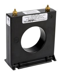
AcuAMP AC current transformer, solid core, 1000A primary, 5A secondary, 2.5in diameter sensing window, 1% accuracy, M4 x 0.7 threaded terminal stud with nut.
