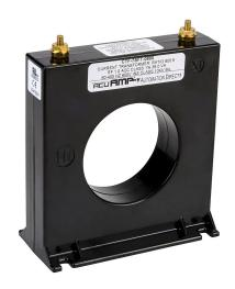
AcuAMP AC current transformer, solid core, 800A primary, 5A secondary, 2.5in diameter sensing window, 1% accuracy, M4  $\times$  0.7 threaded terminal stud with nut.
